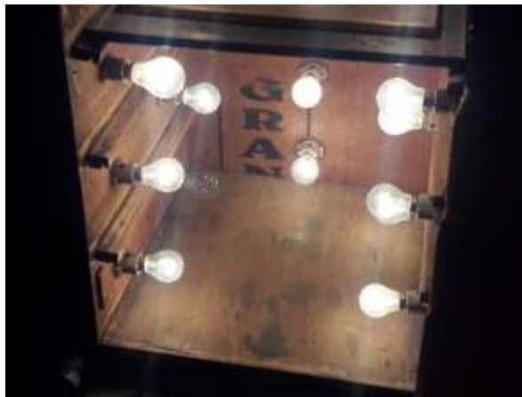
Fig. 1.7.4: Electric bulbs bhatti for drying meena color of payal
