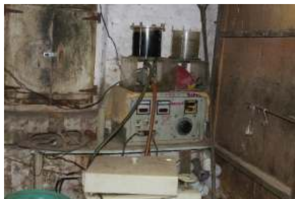
Fig. 1.7.5: Electroplating Vibrator to final polishing of payal
