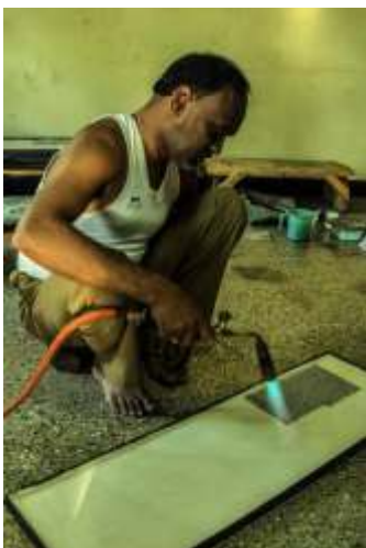
Fig. 1.6.3: Soldering of payal components using flame torch
