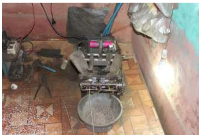
Fig. 1.4.11: Payal components are designed using cutting machine
