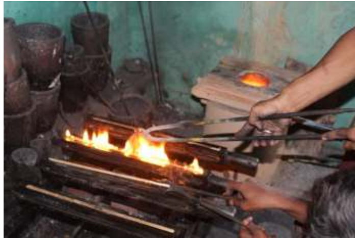
Fig. 1.4.5: Molten Silver being poured in casting frames to form rods
