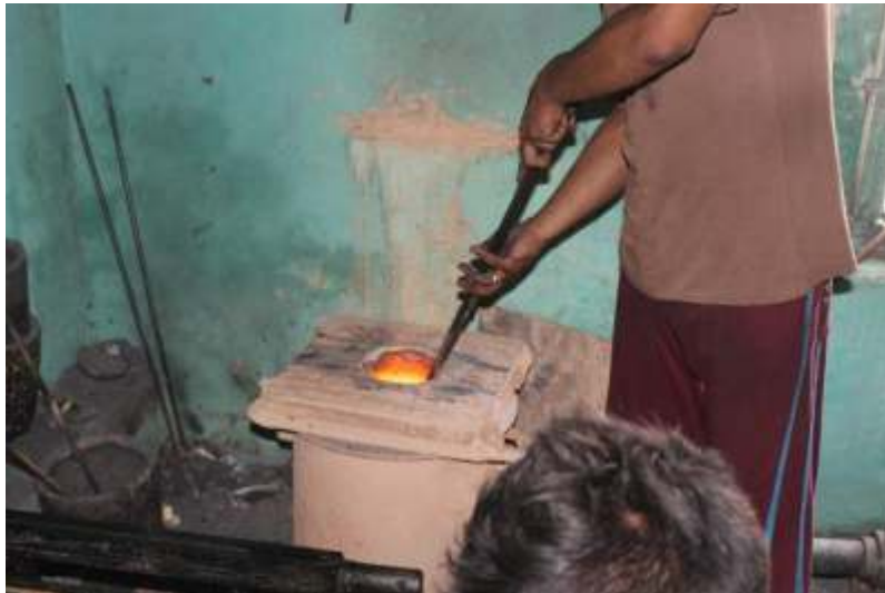
Fig. 1.4.4: Teracotta pot with molten silver is taken out carefully from the furnace
