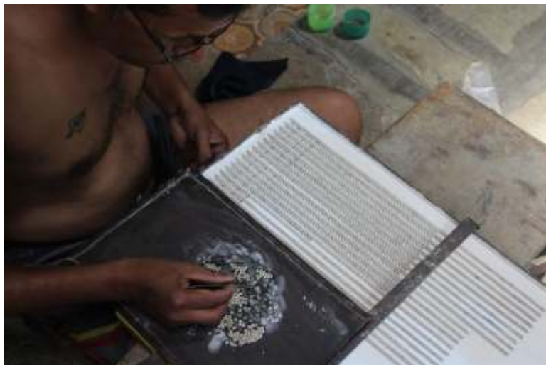
Fig. 1.6.2: Assembling of payal components using soldering solution
