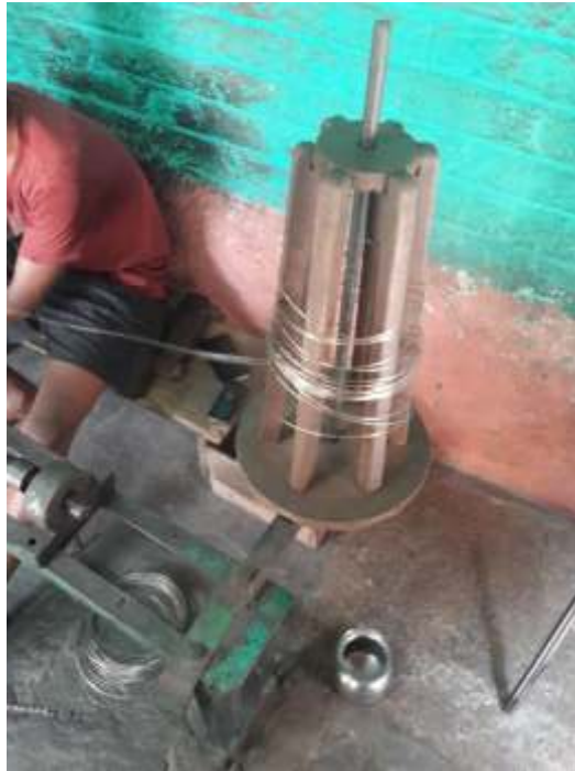
Fig. 1.4.8: Rolling machine to convert silver rods into wires
