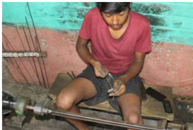
Fig. 1.4.9: Using Gauge Plate to draw silver wires
