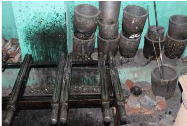
Fig. 1.3.15: Teracotta pots used for heating silver
