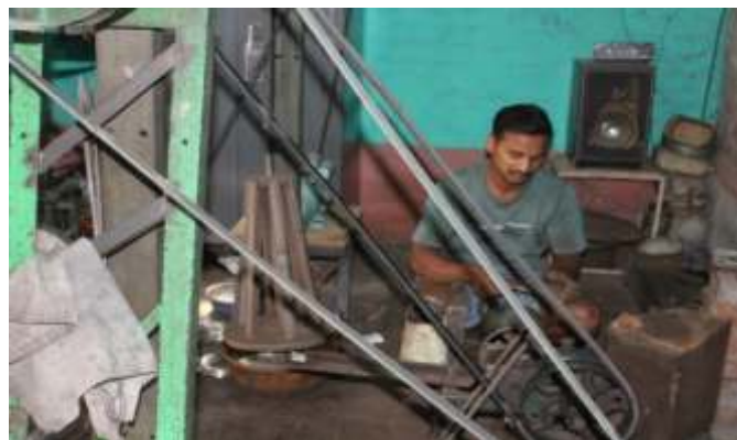
Fig. 1.4.7: Making Silver Wire on roller
